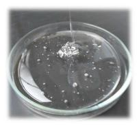
We commercialize water glasses with various molar ratios. Because of its unique properties, water glass is used in a variety of applications, including as a soil hardener for civil engineering, an additive for soap, a chemical for recycling waste paper, and a synthetic raw material for silica gel and zeolite.
